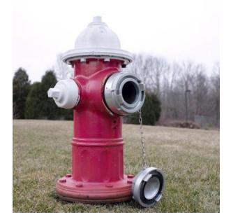
The Hydrant Storz adapters permanently change main hydrant outlet from threads to Storz. This picture Includes hard anodized adapter and cap with chain and stainless steel set screws to prevent unscrewing from the hydrant.
